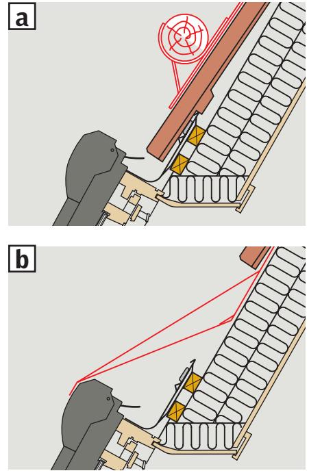
**ENGLISH:** As a precondition to avoiding any damage to the roller shutter in very cold regions and in regions with heavy snowfall, either a snow-wedge or a snow stop must be installed above the roller shutter **a**, **b**. In case of snow on the roof, care must be taken when operating the roller shutter.
